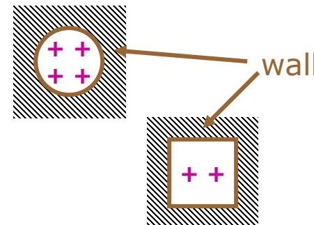
Artefacts, severe distortion of properties near the wall → mainly due to wrong short range forces
