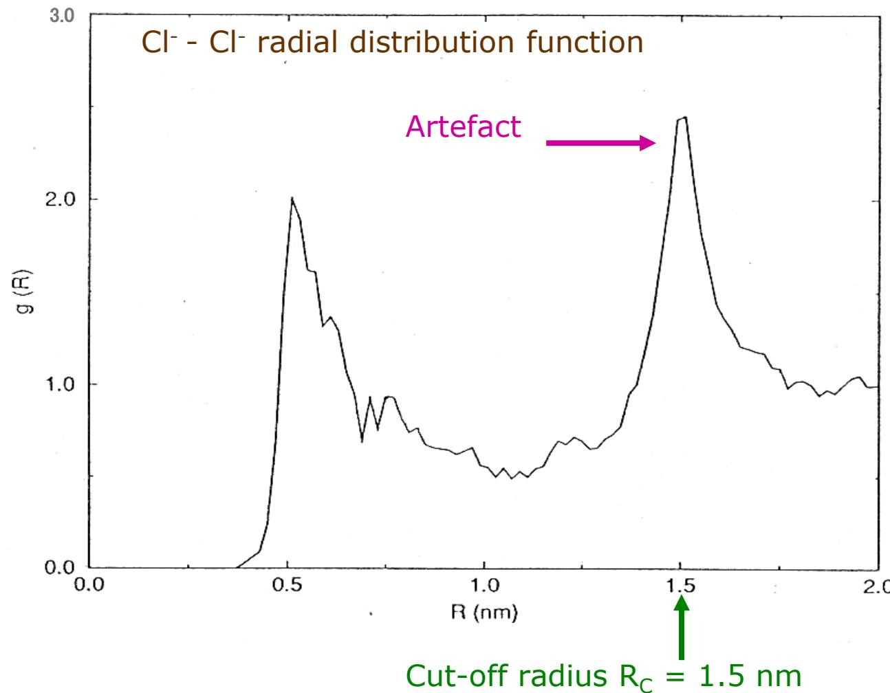
Cut-off distortion is present, even for long cut-off distances
